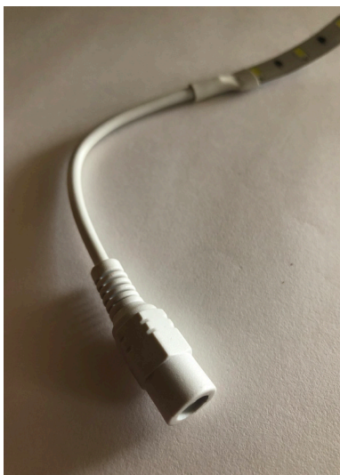
The lights run on 12V DC and come with a female barrel connector pre-wired at one end
